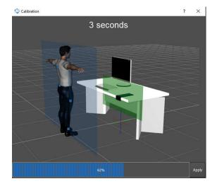
It is always recommended to calibrate the system at the start of each recording. If you want to make more recordings on the subject without repeating the calibration phase every time, it is recommended to Reposition the system using the Reposition button.
