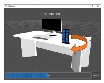
Rotate the base on the sagittal plane by 90 ° so as to observe the LEDs of the sensors from above
