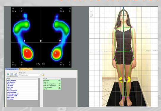
Plantar pressure loads shown in 3D, high resolution and numeric values. 250 frames captured over a period of 5 seconds. Lateral/Medial and Rear/Forefoot pressure distribution, surface area, center of pressure calculations with automatic report.
