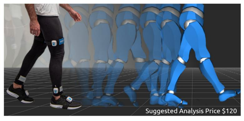
MOVIT is using 7 IMU sensors that allow to capture the real body motion during the walking with a real 3D animation. It generates an automatic report showing all the spatio-temporal parameters, symmetry indeces, joint angles of pelvis, hip, knee and ankle. Also used with synchronized camera.
